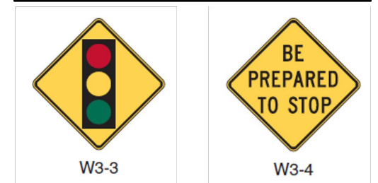
W3-3 "Signal Ahead" with W3-4 "Be Prepared to Stop", from the MUTCD - S13
