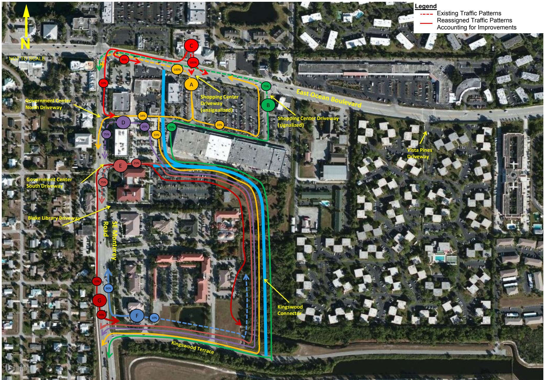
Figure 12 Traffic Reassignment East Ocean Boulevard/SE Monterey Road Martin County, Florida
