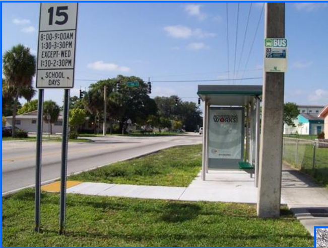
Sidewalk should be provided from edge of travel lane and connect to bus stop/shelter and sidewalk network
