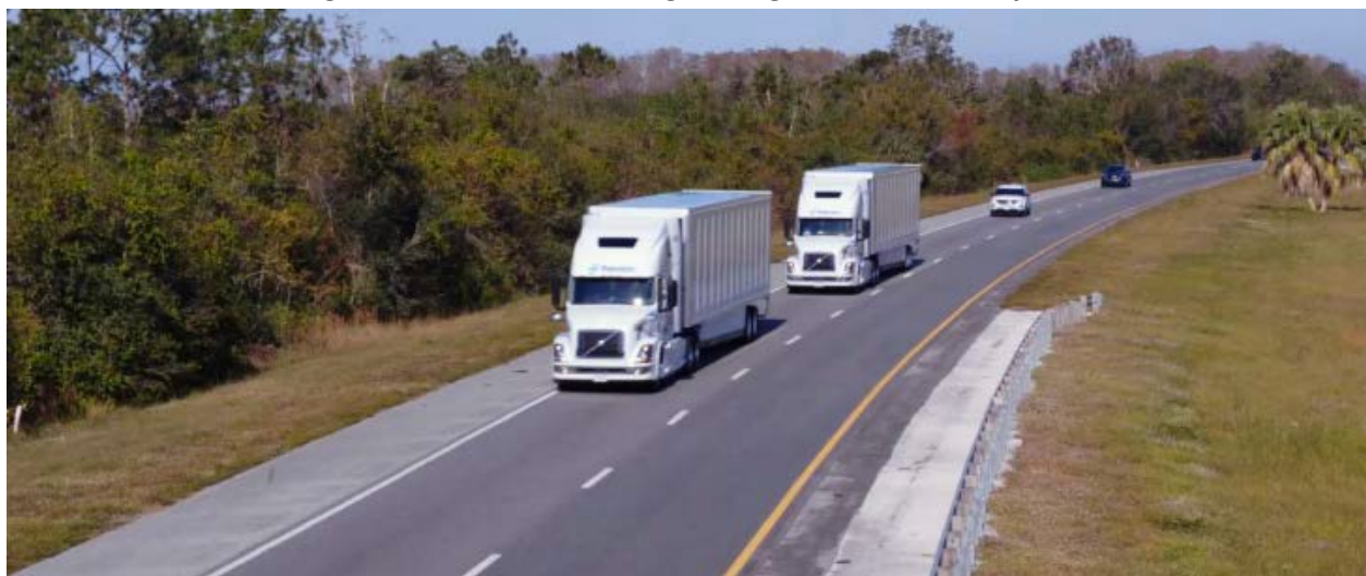
Figure 6.2 - Truck Platooning Testing on Florida's Turnpike
