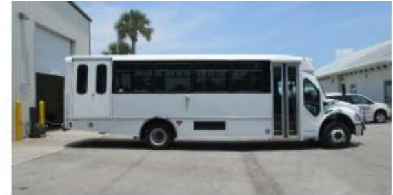
Length: 29+ ft. Passengers: 20-24 Chassis: Medium-duty or Light-duty
