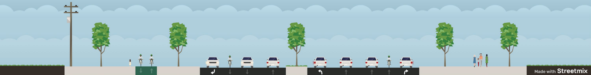
15' Pathway for Bicycles & Pedestrians (West Side) and 10' Shared Use Pathway (East Side)
