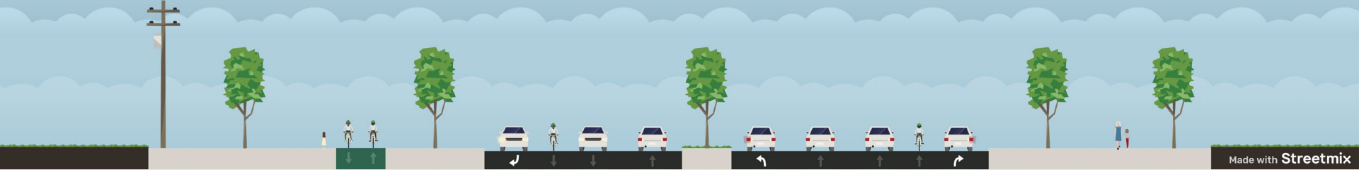
15' Pathway for Bicycles & Pedestrians (5' Sidewalk with 10' Two-Way Bikeway – West Side), 6' Sidewalk (East)
