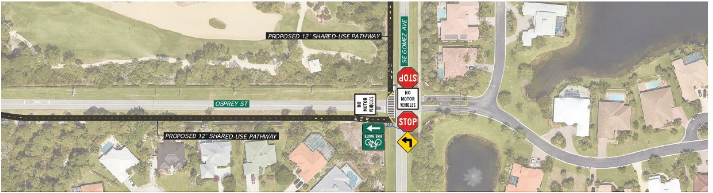
Figure 66: Conceptual Plan View (SE Osprey Street to SE Gomez Ave)
